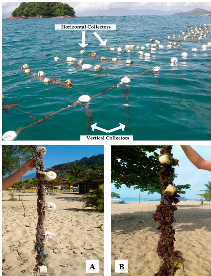
Figure 1. Sixteen collectors positioned horizontally at the surface of the sea at the air-water interface and another 16 positioned vertically underneath the water surface. (A) collector before deployment at the sea, (B) collector after immersion time with organisms already settlement.
